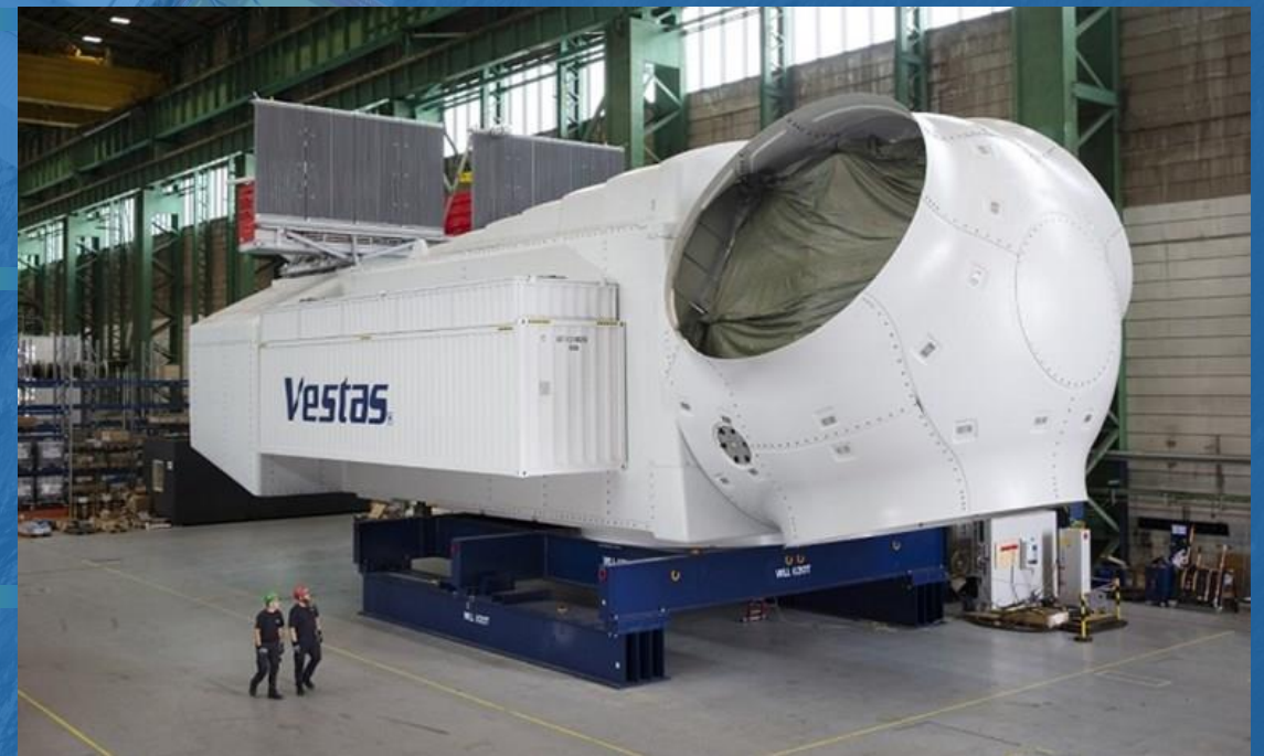
The nacelle of the V236-15.0MW turbine that will be assembled at the Szczecin plant
