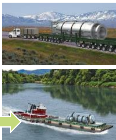
NPM pressure vessel & component transportation to site
